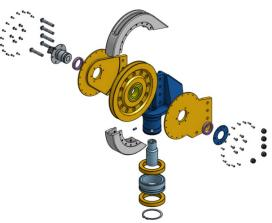
The sheave spins on an AST 5308-2RS 40mm ID Double Row, angular contact, deep groove ball bearing which provides excellent wobble stability and high load carrying capacity. All bearings are loaded below their fatigue limit (Pu) so life should be nearly infinite.
