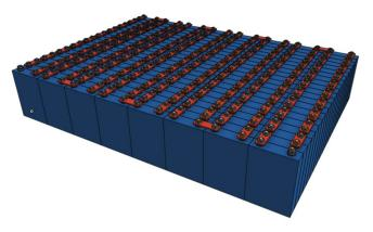
The Remy HVH 250-115 and its John Deere PD400 inverter can use as much as 900VDC but will still work down to 180V. A 538VDC pack is a compromise judged adequate for the expected duty.
