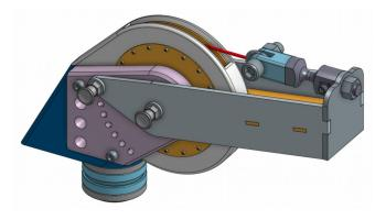
they stay greased, clean and ready for use. The blade can easily cut through both the plastic tube and rope.
