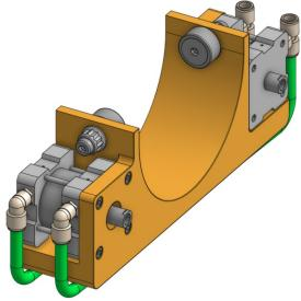
**Drive Line Component - Brake:** Traditionally, glider winches have used friction brakes – usually a drum. This brake has two purposes - to stop the drum in an emergency and to provide rope tension as the ropes are pulled back to the start line.
