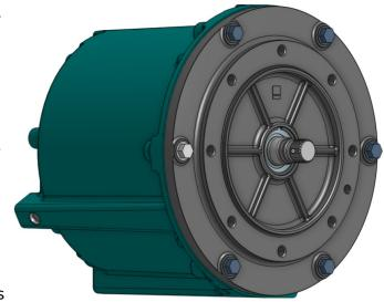
The HVH250 is a liquid cooled, 3-phase AC Permanent Magnet Synchronous Motor (PMSM) with no brushes or slip rings. The only moving part is the rotor which contains the magnets. It is driven by a variablefrequency traction inverter.
