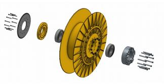
Each drum rides on large ball bearings which allows the shaft to rotate inside a stationary drum – or the drum to rotate on a stationary shaft. The bearing nearest the dog clutch is 75mm ID and the bearing nearest the ends of the shaft is 70mm ID to make it easier to mount on the stepped shaft.
