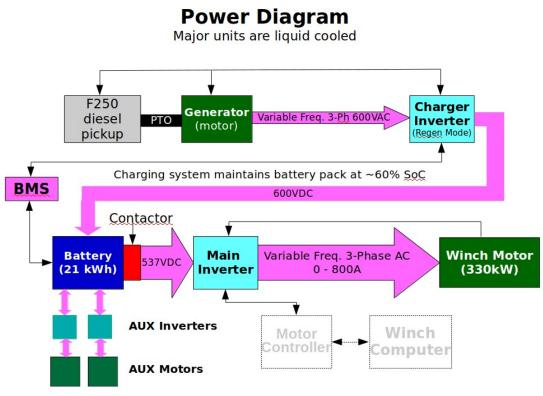
Thin black lines are signal wires
