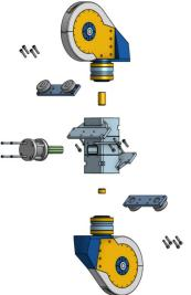
After bending around the top sheave, the rope travels vertically downward through the bollow axis of the caster "wrist" bearings, through
