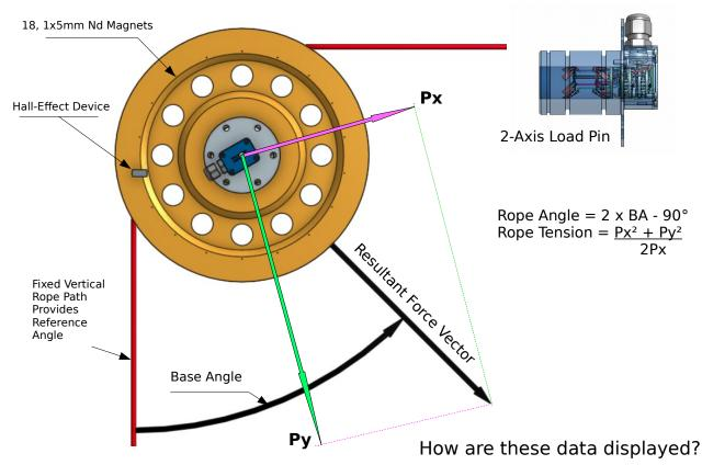
A winch operator – or winch computer - needs five real-time data streams. These are rope tension, rope elevation angle, rope speed, rope length remaining plus environmental data such as wind and temperature. Sensors on the fairlead provide the first four as shown above.
